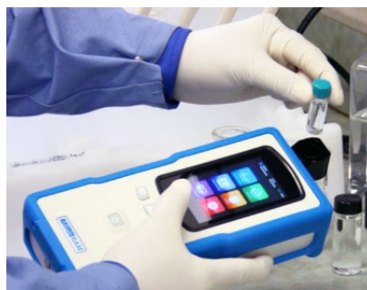
Image no. 2. Spectroscopic scanning a drug vial.
