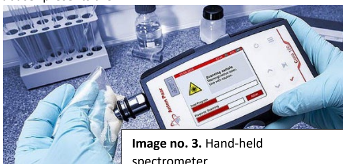
Image no. 2. Spectroscopic scanning a drug vial.
