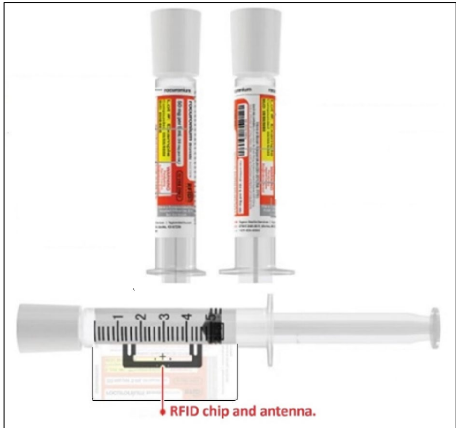
Image no. 12. Adhesive label with an RFID tag attached to syringes. The actual RFID chip is very small and its associated antenna is thin enough to be rolled around the syringe. The label can also be designed to be attached, sticking out to the syringe's side, like a flag. That spares covering the syringe volume markings.
